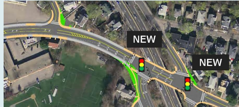
The project includes new and enhanced pedestrian crossings at several locations, including both sides of the Route 9 intersection (shown above), as well as at two realigned intersections - Oak St/Christina St and Charlemont St.
